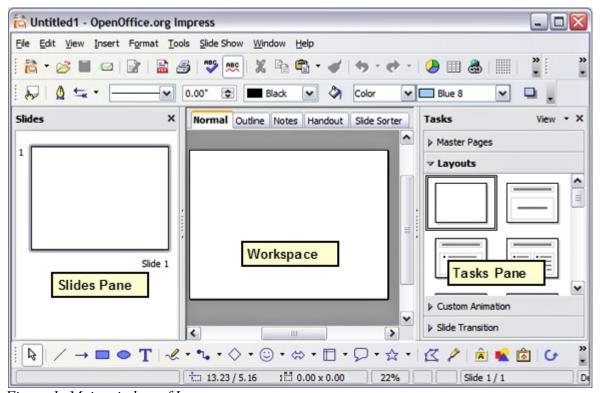
Figure 1: Main window of Impress
