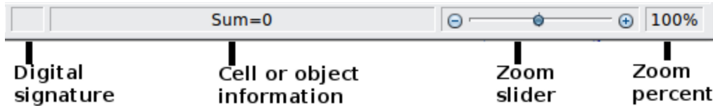
Figure 6: Right end of Calc status bar
