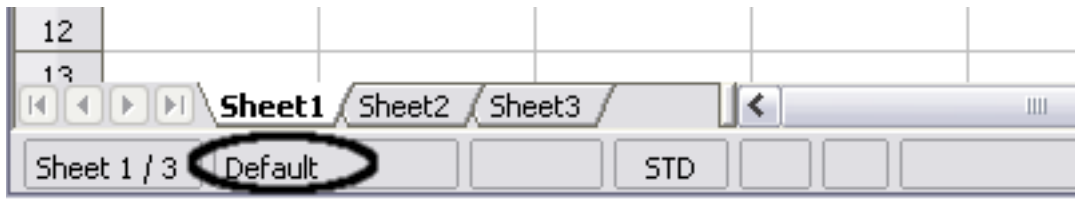
Figure 99: Status bar showing location of page style information below the sheet tabs.
