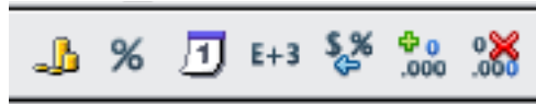
Figure 16: Number format icons. Left to right: currency, percentage, date, exponential, standard, add decimal place, delete decimal place.
